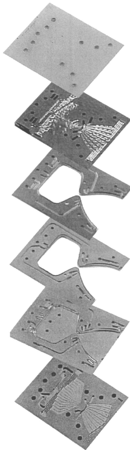
Fig. 10 Thrust chamber and nozzle consists of six wafers.
